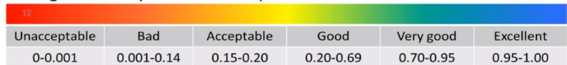
Orthogonal Quality mesh metrics spectrum
